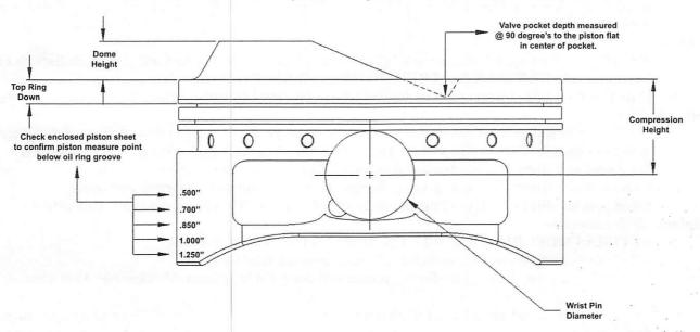
Piston to bore clearance on enclosed piston spec card is referenced as a miniumum setting. Refer to chart below for specific application adjustments to piston to wall clearances.
